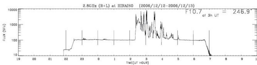
**Fig. 14** Example of a series of radio wave bursts that occurred in December 2006 and affected GPS positioning precision
