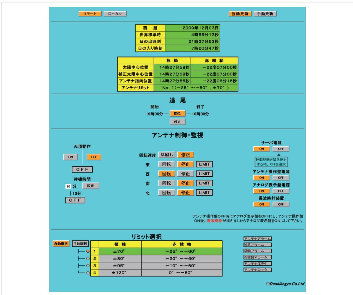
Fig. 12 Webpage for controlling a 10-meter antenna
