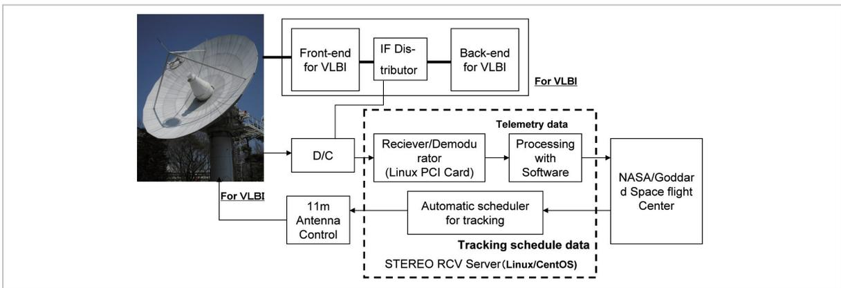
**Fig.3** Conceptual diagram of the STEREO reception system additionally arranged with the backend of VLBI observation equipment
