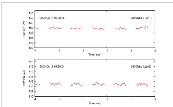
**Fig. 11** 2.8 GHz solar radio waves observed with high time resolution of 0.5 to 1 millisecond
