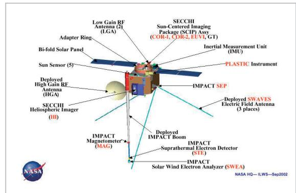
**Fig. 2** External view of the STEREO spacecraft
