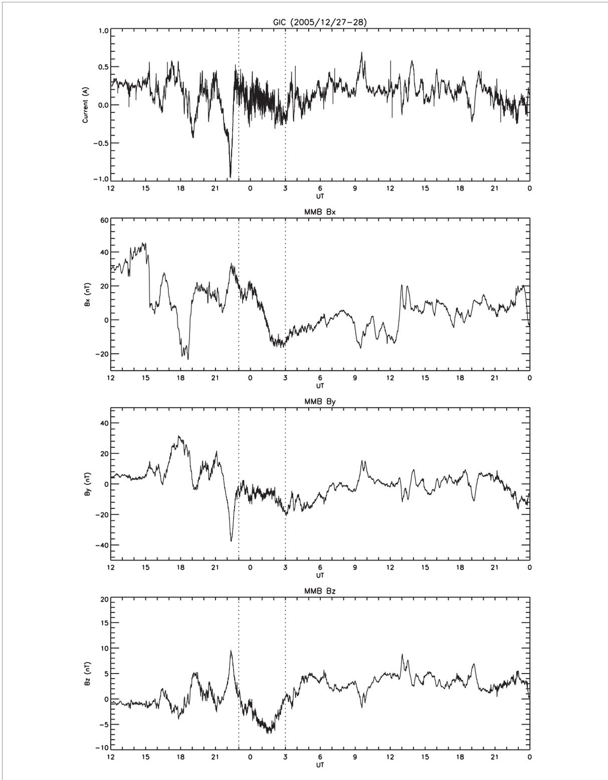
**Fig.7** An example of GIC due to geomagnetic pulsations
