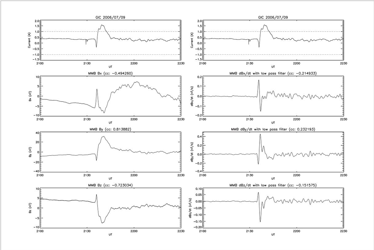
**Fig.5** An example of GIC stemming from an impulsive change in the geomagnetic field due to an interplanetary shock
