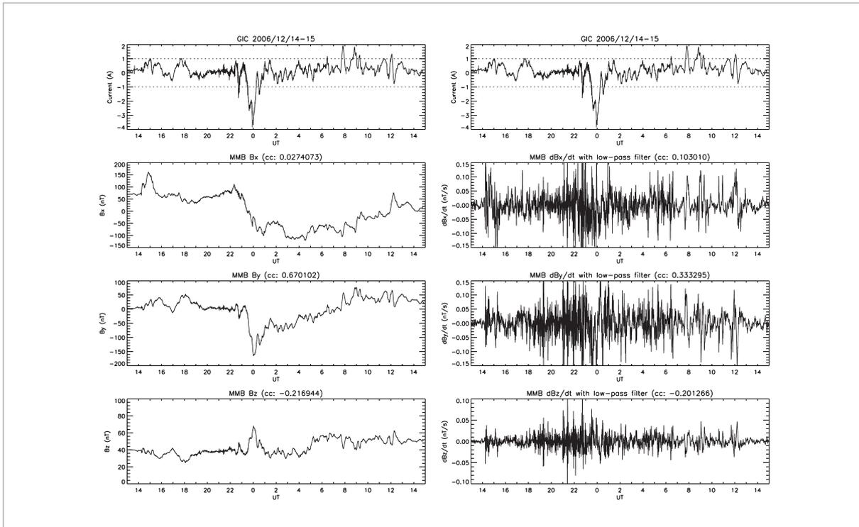
**Fig.4** An example of GIC stemming from a geomagnetic storm
