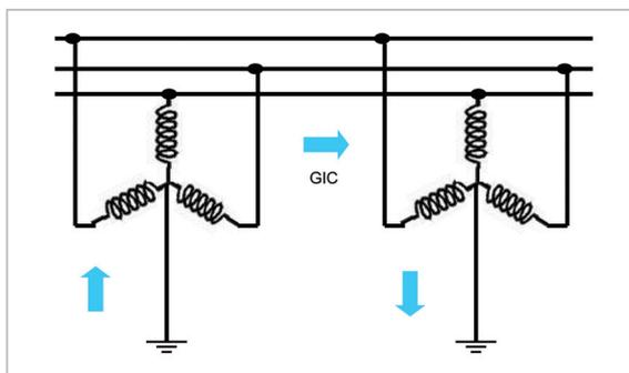
**Fig. 1** Geomagnetically induced current (GIC) flowing through an electric power grid due to variations in the geomagnetic field
