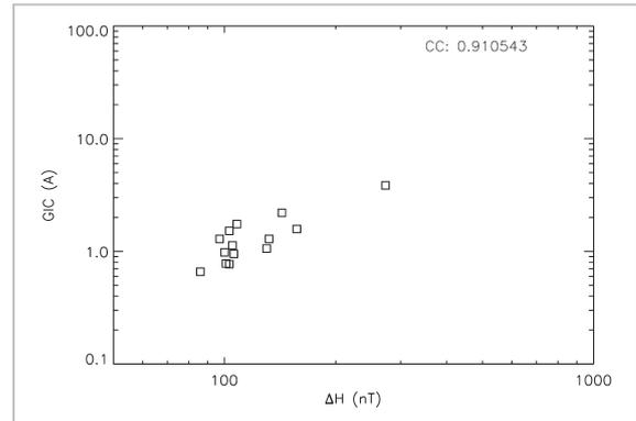
**Fig.8** A plot of maximum variations in the horizontal component ( $\Delta H$ ) at the time of the geomagnetic storms listed in Table 2 and maximum values of corresponding GIC
