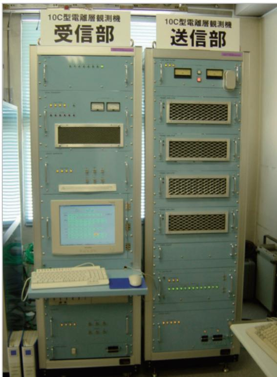
Fig.2 10C type ionosonde transceiver
