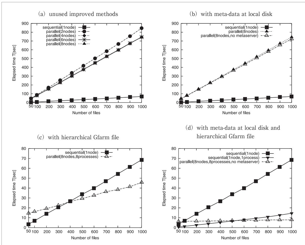
**Fig.5** Comparison of processing time for distributed parallel processing of GEOTAIL/orbit data with sequential processing
