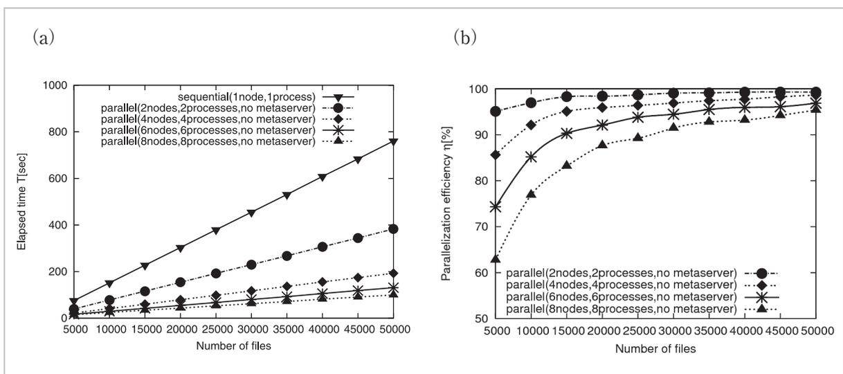
**Fig. 7** Comparison of distributed parallel processing of GEOTAIL/orbit data (using meta-data local caching and hierarchical segment files) with sequential processing
