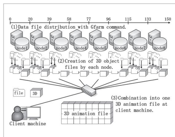
**Fig. 8** Distributed parallel processing for visualization
