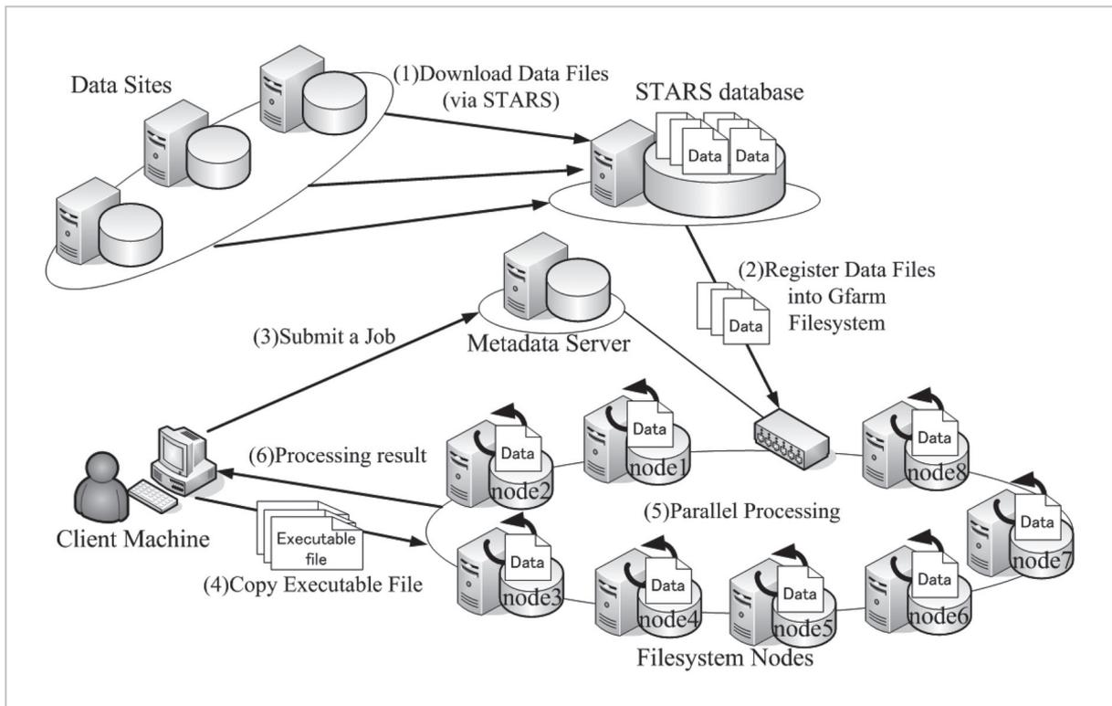
**Fig. 1** Parallel distributed processing system running on STARS and Gfarm
