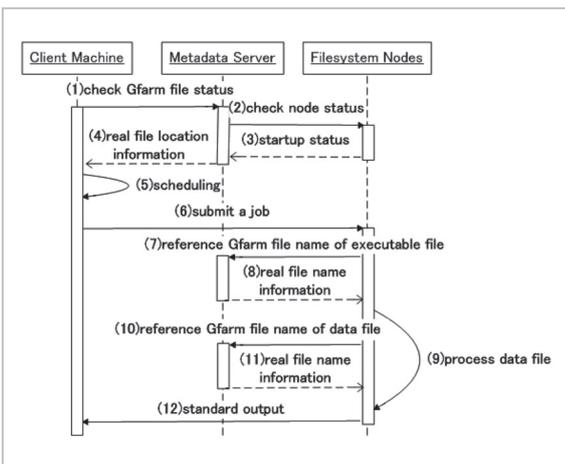
**Fig.3** Flow of distributed parallel processing on Gfarm
