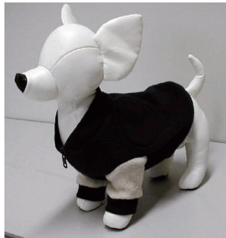
Fig. 3 Example of pet clothing attached with an antenna
