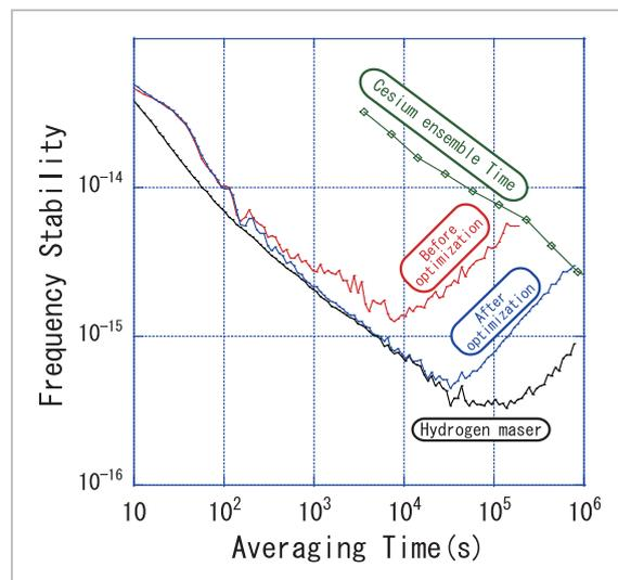
**Fig.9** Frequency stabilities of the source clock Hydrogen Maser, TA and UTC(NICT) before and after parameter optimization
