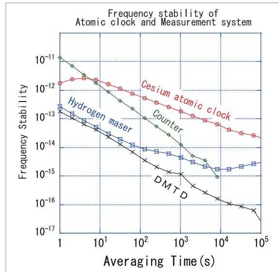
**Fig.2** Frequency stabilities of source clocks and measurement systems
