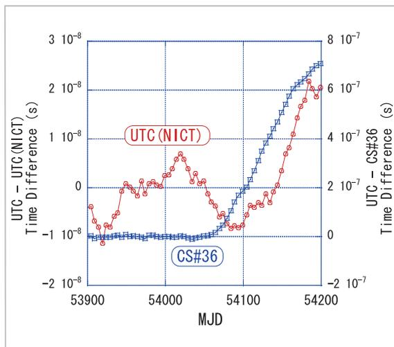
**Fig.4** Time differences between UTC, UTC(NICT) (left vertical axis) and CS#36 (right vertical axis) evaluated from Circular T
