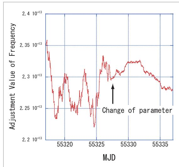
**Fig.8** Time-series data of adjusted frequency values for the actual system before and after parameter optimization
