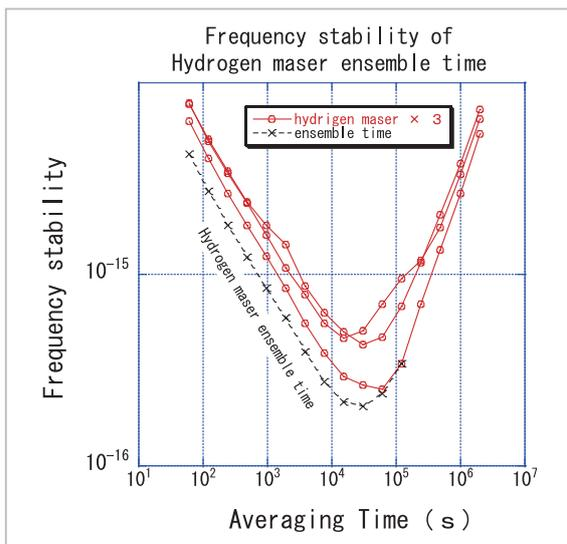
**Fig.10** Frequency stabilities of the ensemble atomic time using three hydrogen masers and each of three hydrogen masers
