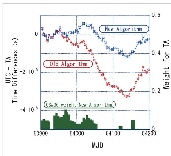
**Fig.5** The weight of CS#36 for new algorithm, and the time differences between UTC and TA produced by the former and new algorithms
