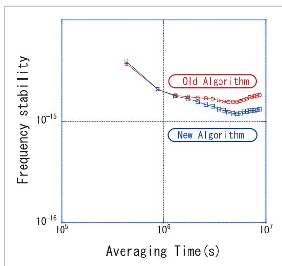
**Fig.6** Frequency stability of UTC-TA before and after improving algorithms
