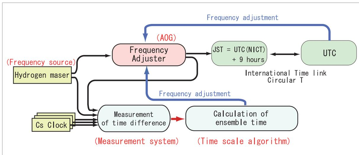
Fig.1 Basic configuration of the JST system
