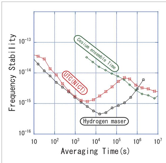
**Fig.7** Frequency stabilities of the source clock hydrogen maser, TA and UTC(NICT) for 2007/2/1~2010/7/27 (long-term) and 2009/2/1~2009/7/27 (~midterm)
