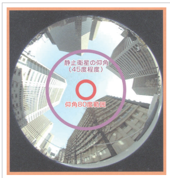
Fig.3 Example for optimal orbit; difference in vision between a geostationary satellite and a QZS from an urban canyon
