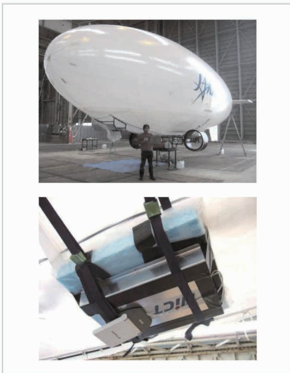
Fig.53 Test on collection of damage information by LTA aircraft
