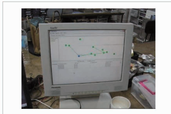
Fig.41 Screen of ad hoc network topology
