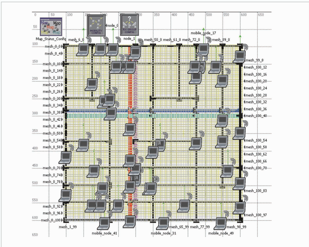
Fig.29 Terminal traveling model in the area, simulating the central area of Sendai City
