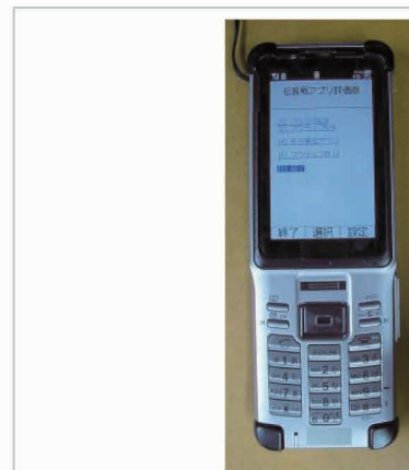
Fig. 130 Ubiquitous terminal containing UHF-band passive/active RFID reader/writer and the screen of message board application
