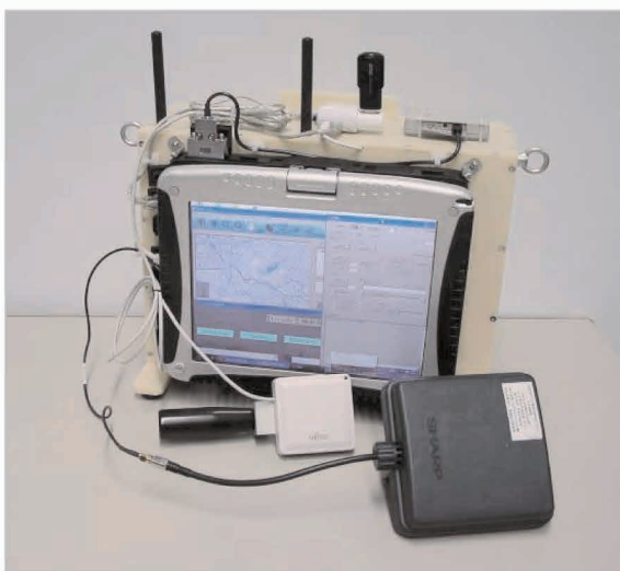
Fig. 142 Integrated multi-RFID reader/writer
