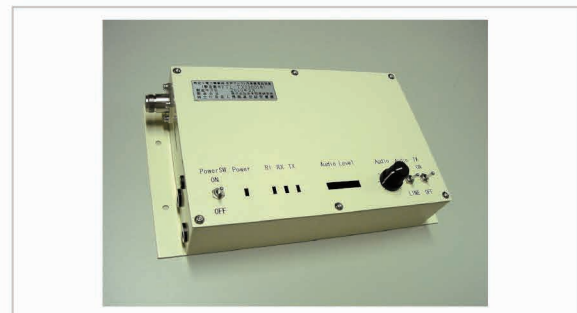
Fig. 145 Prototype radio telephone equipment for voice assistance
