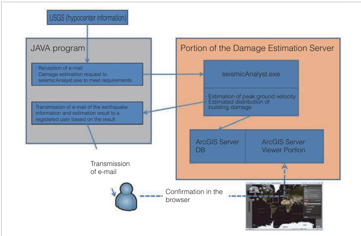
**Fig.7** Configuration of the international version of the Simplified Earthquake Damage Estimation System and the flow of information
