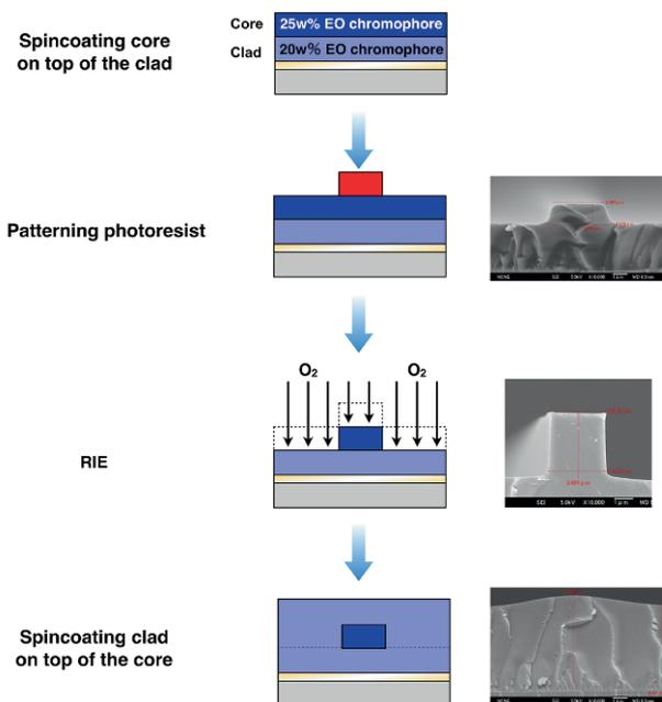
Fig. 5 Fabrication process of all EO polymer optical waveguide structure
