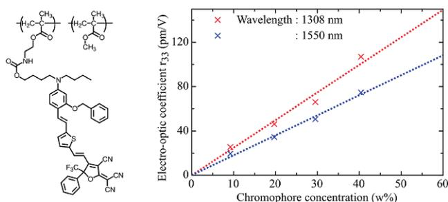
**Fig. 4** (a): Structure of a side chain polymer and (b): Dependence of the electro-optic coefficient on the concentration of chromophores
