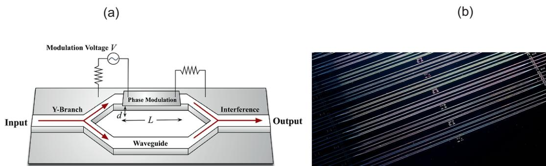
Fig. 1 (a): Schematic diagram of a MZ interferometer and (b): MZ optical waveguides fabricated on Si wafer
