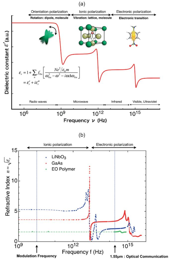
**Fig. 2** (a): Types of dielectric polarization and (b): Wavelength dispersion of refractive indices of typical electro-optic materials
