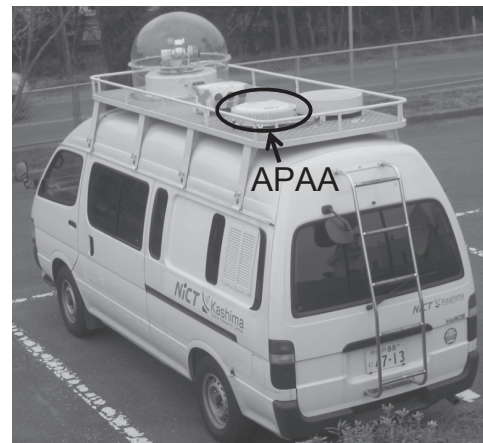
Fig. 4 Appearance of the antenna on the vehicle
