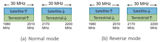
Fig. 1 Satellite/terrestrial frequency sharing method
