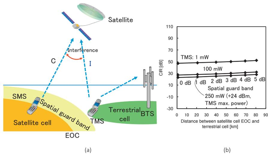
**Fig. 5** Interference paths and evaluation: normal mode satellite up-link
