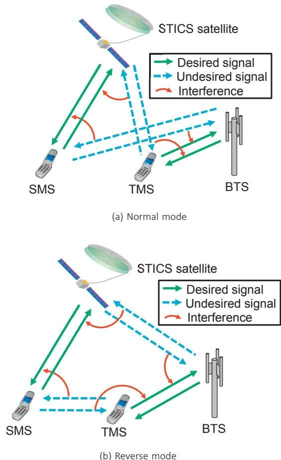
Fig. 3 Satellite/terrestrial interference paths
