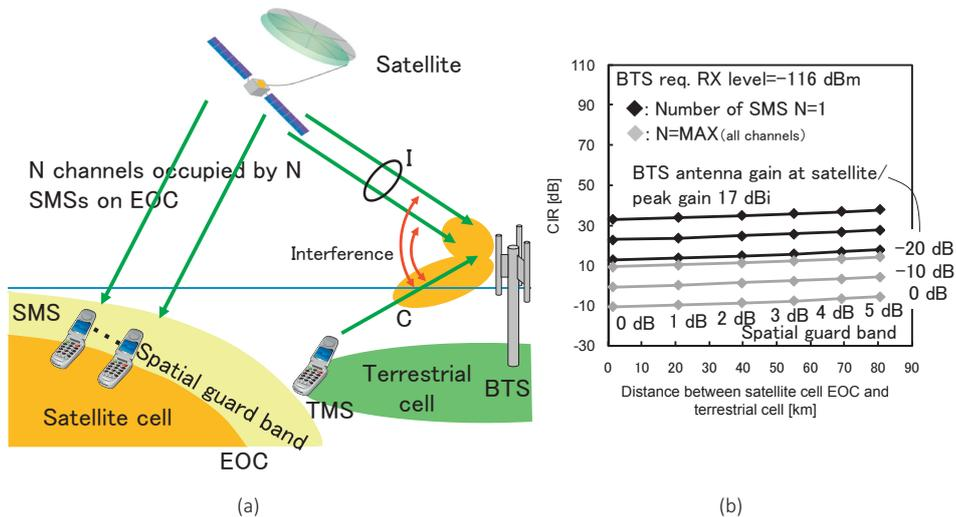
Fig. 11 Interference paths/evaluations: reverse mode terrestrial up-link
