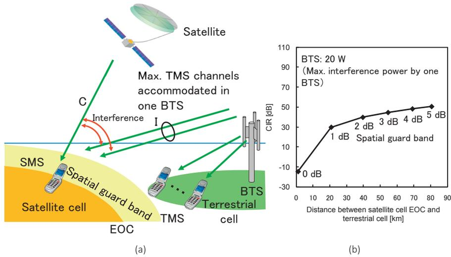
Fig. 6 Interference paths and evaluations: normal mode satellite down-link
