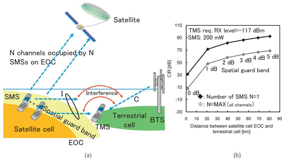
Fig. 12 Interference paths/evaluations: reverse mode terrestrial down-link
