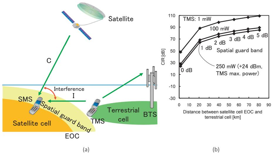
Fig. 10 Interference paths/evaluations: reverse mode satellite down-link
