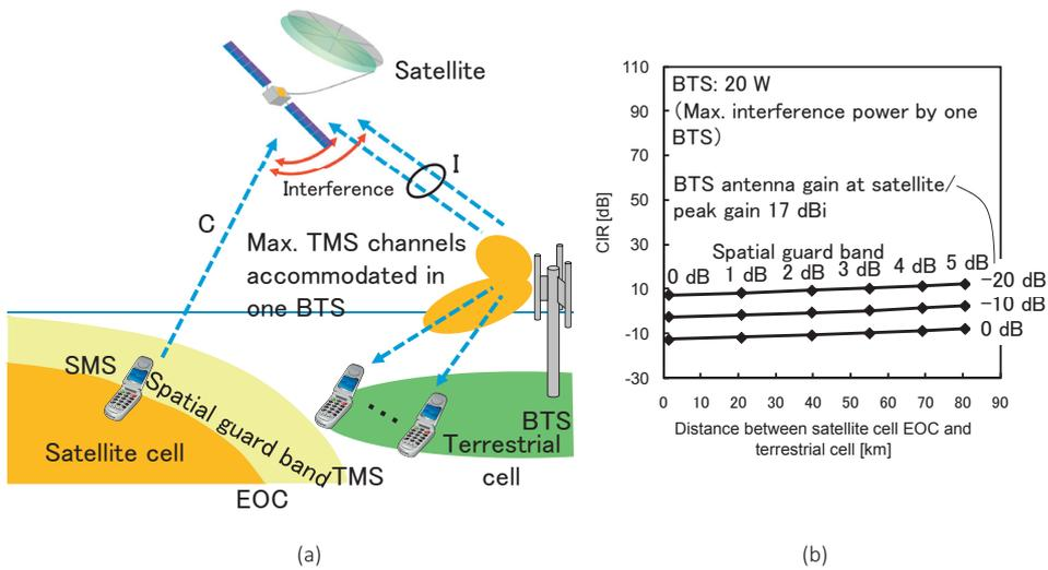
Fig. 9 Interference paths/evaluations: reverse mode satellite up-link
