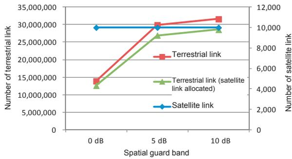
Fig. 15 Number of links simultaneously accommodated when satellite up-link established
