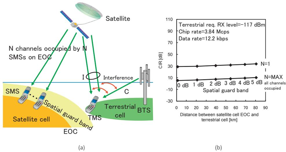
Fig. 8 Interference paths/evaluations: normal mode terrestrial down-link
