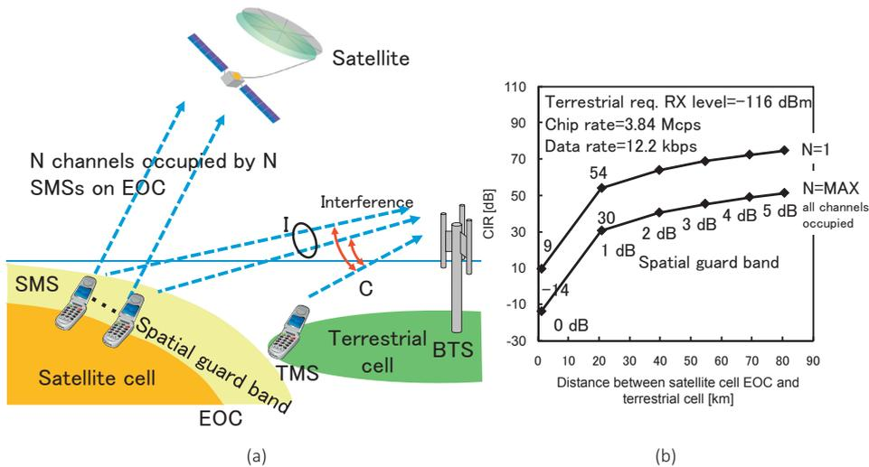
Fig. 7 Interference paths and evaluations: normal mode terrestrial up-link
