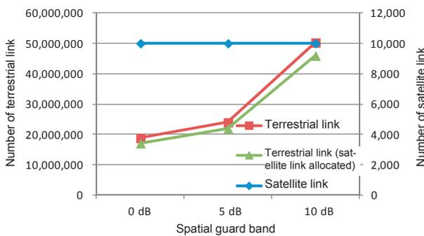
Fig. 16 Number of links simultaneously accommodated when satellite up-link established in disaster situation
