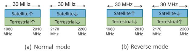
Fig. 1 Satellite/terrestrial frequency sharing method
