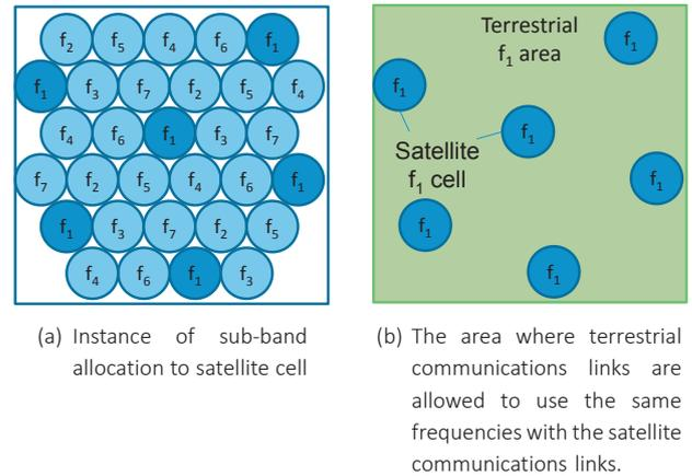
Fig. 2 Scheme of frequency sharing (7-cell repetitive use for a satellite cell)
