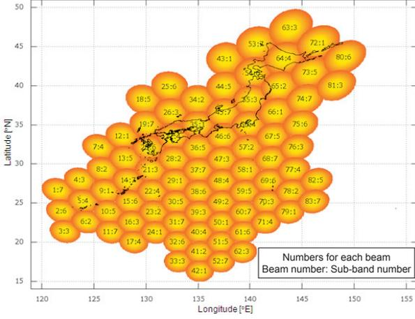
Fig. 14 Satellite beam configuration
