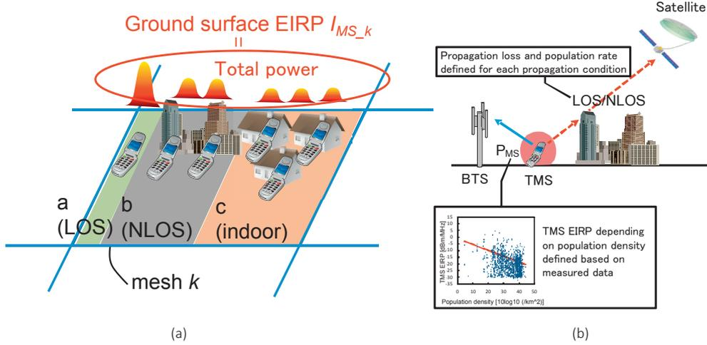
Fig. 13 Interference model for satellite terminal: schematic diagram
