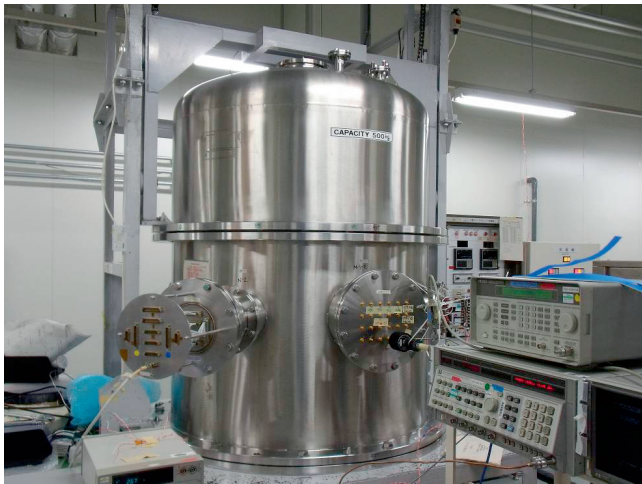
Fig. 24 Thermal vacuum test setup (center: vacuum chamber)
