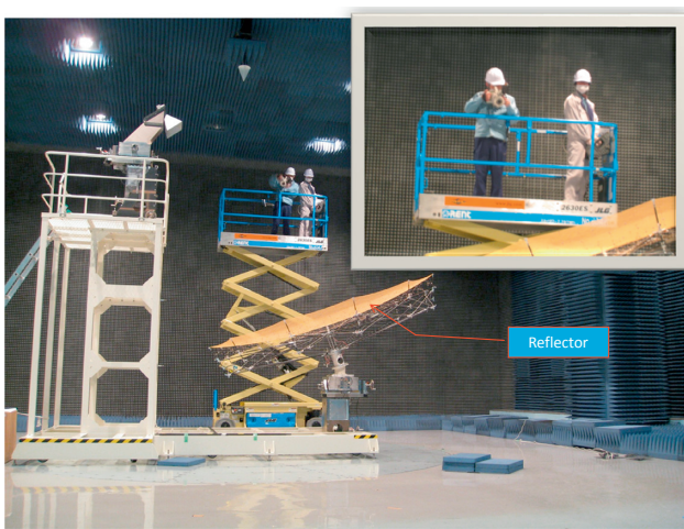
Fig. 5 Measurement of reflector shape
