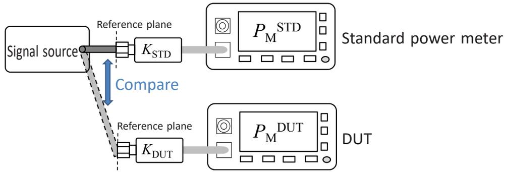
Fig. 2 Power meter calibration by comparison method
