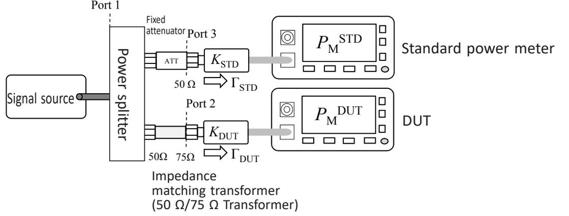
Fig. 4 Power meter calibration by simultaneous comparison method
