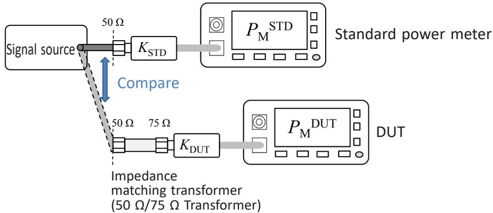
Fig. 3 Comparison method using an impedance matching transformer (50 Ω/75 Ω)
