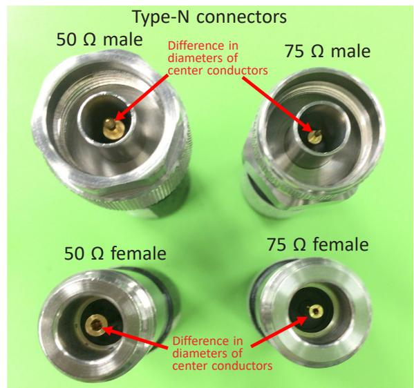
Fig. 7 Shapes of type-N coaxial connectors
