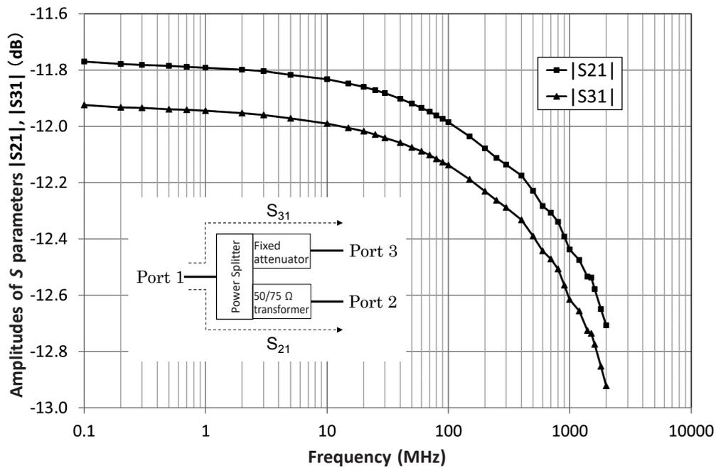
Fig. 8 Power splitter's  $S$  parameters measurement results example
