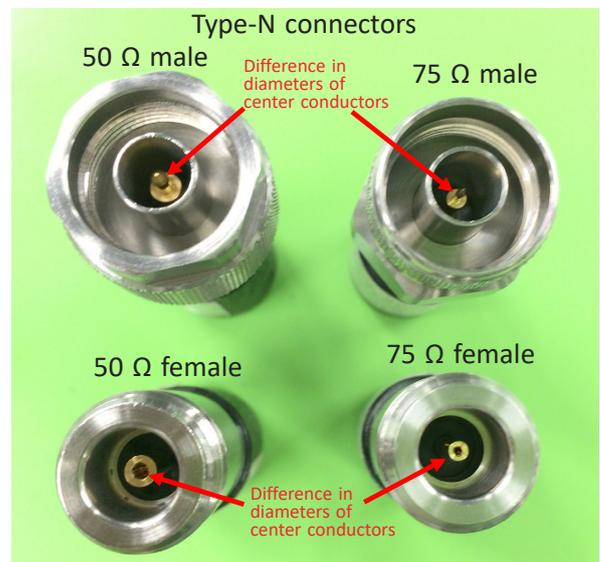
Fig. 7 Shapes of type-N coaxial connectors
