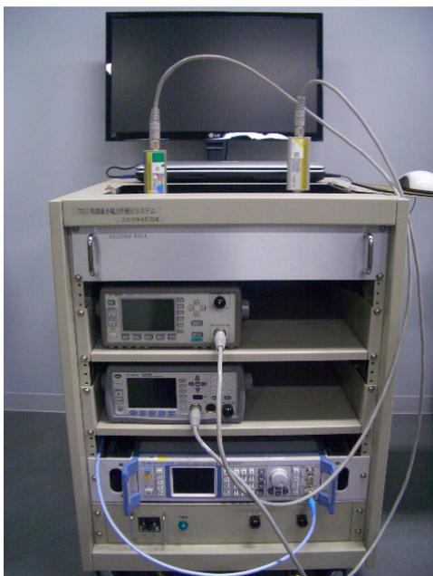
Fig. 6 High frequency power meter calibration system (1 mW, 75 Ω) photo
