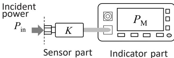
Fig. 1 Configuration of high frequency power meter
