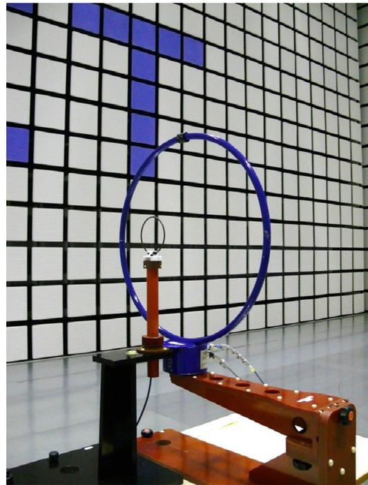
Fig. 2 Configuration to calibrate a loop antenna
