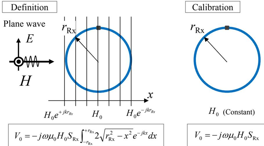
Fig. 7 Unevenness of magnetic field that interlinks with the loop area
