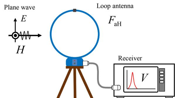
Fig. 1 Magnetic field measurement and definition of magnetic field antenna factor
