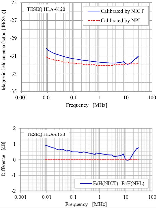
Fig. 5 Calibration results example (Teseq, HLA-6120)
