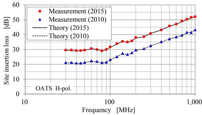
Fig. 8 SIL measurement results at OATS (Horizontal polarization)
