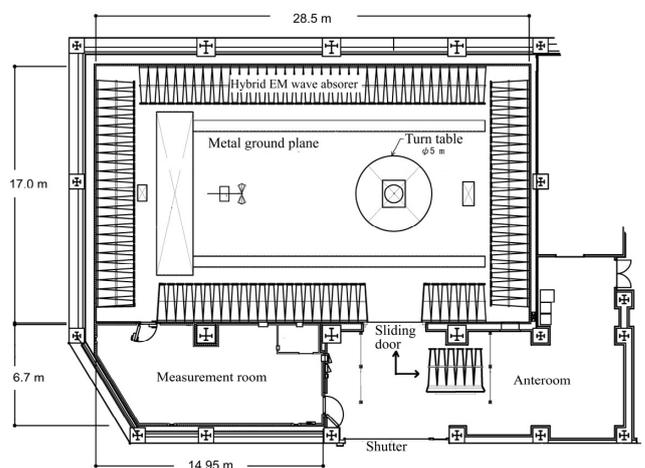
**Fig. 5** Ground plan of Semi-Anechoic Chamber (SAC)
