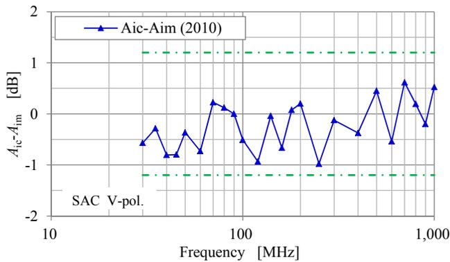
Fig. 16 Differences of SIL between theoretical and measurement values at SAC (Vertical polarization)
