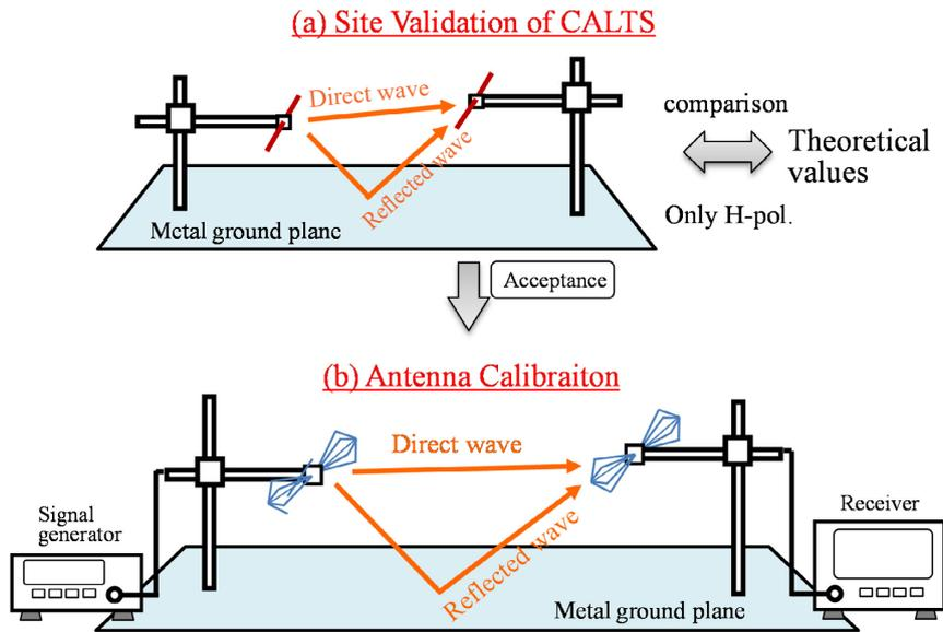
Fig. 6 Calibration of antenna for EMI measurements
