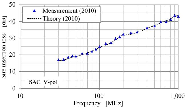
Fig. 15 SIL measurement results at SAC (Vertical polarization)
