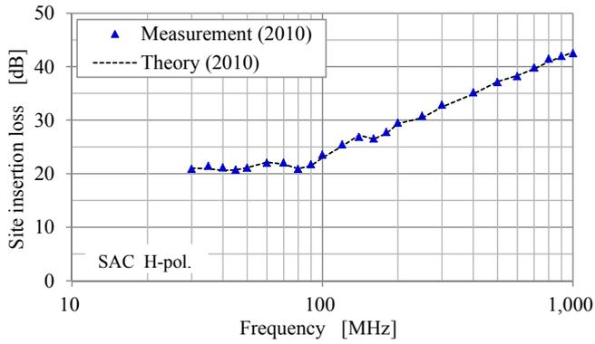
Fig. 13 SIL measurement results at SAC (Horizontal polarization)
