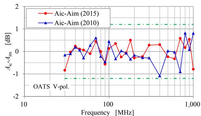
Fig. 11 Differences between theoretical values and SIL measurement results at OATS (Vertical polarization)
