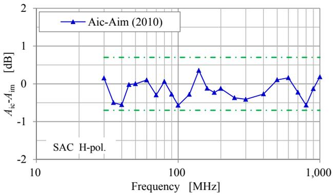
Fig. 14 Differences of SIL between theoretical and measurement values at SAC (Horizontal polarization)
