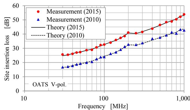
Fig. 10 SIL measurement results at OATS (Vertical polarization)
