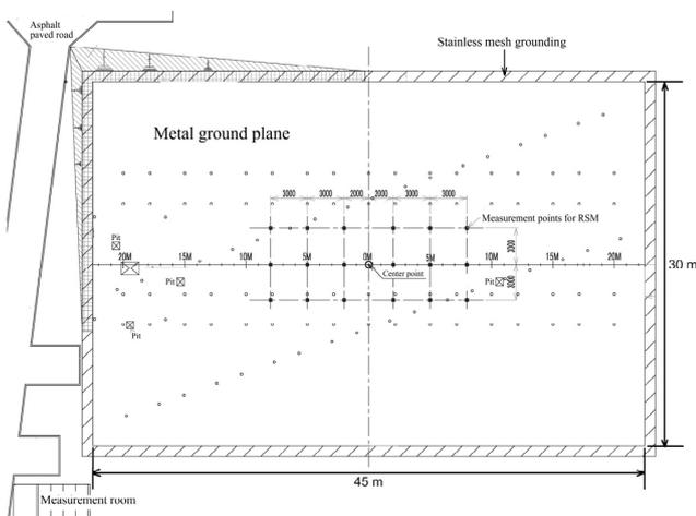
**Fig. 3** Ground plan of Open Area Test Site (OATS)
