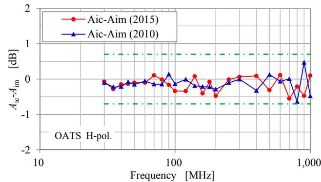
Fig. 9 Differences between theoretical values and SIL measurement results at OATS (Horizontal polarization)
