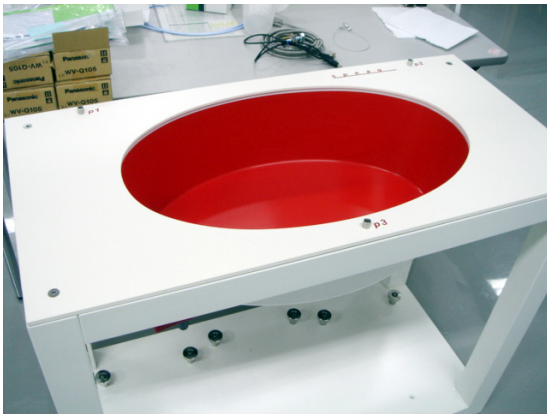
Fig. 3 Flat phantom (Elliptical Shape)
