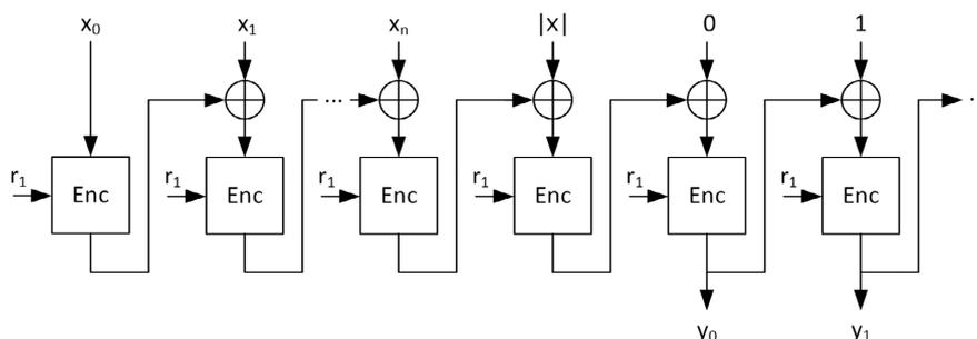
Fig. 2 Pseudorandom function that uses symmetry key encryption
