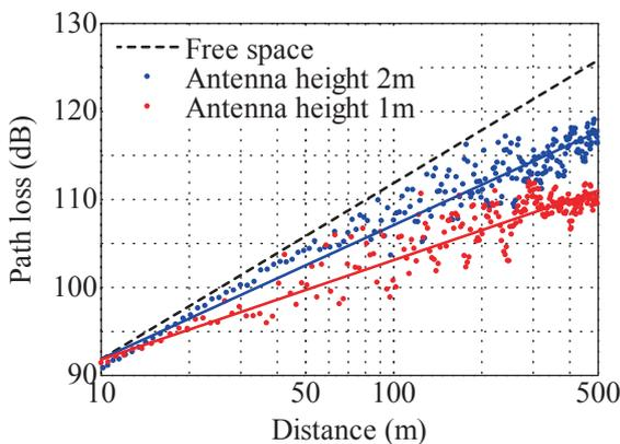
Fig. 3 Path loss characteristics in 90 GHz band (Measured with vertical polarized signal) (Copyright(C)2017 IEICE, [2] Fig. 5)
