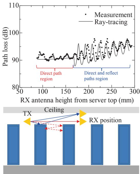
Fig. 12 Validation of measurement result by ray-tracing method
