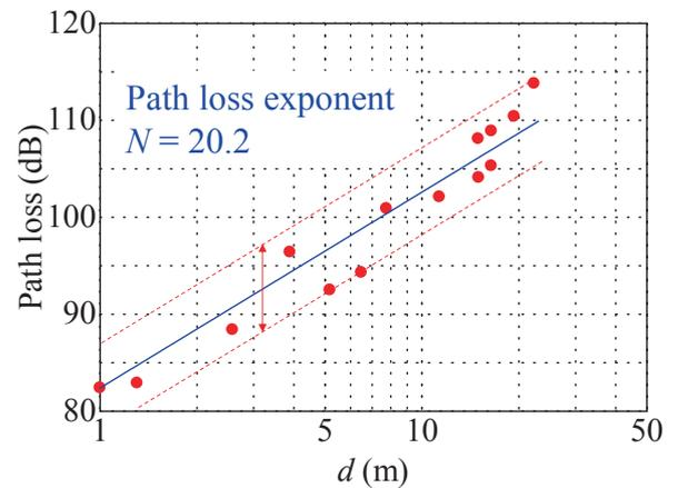
Fig. 11 Path loss measurement results in data center environment (Copyright(C)2017 IEICE, [4] Fig. 5)
