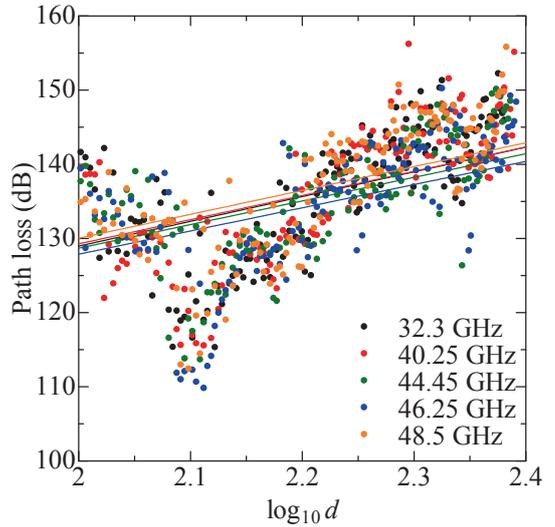
**Fig. 8 Path loss measurement results in NLoS urban environment**
