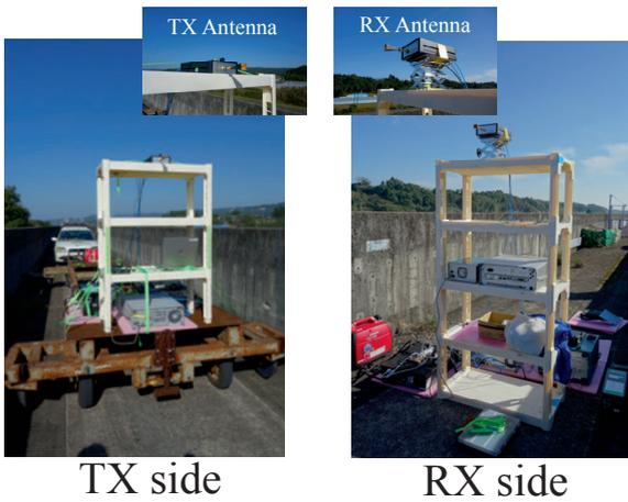
Fig. 1 Propagation measurement in viaduct environment (Copyright(C)2017 IEICE, [2] Fig. 4)
