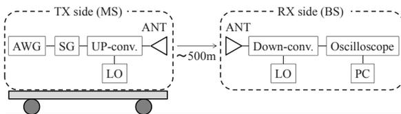
Fig. 2 Propagation measurement system in 90 GHz band (Copyright(C)2017 IEICE, [2] Fig. 4)
