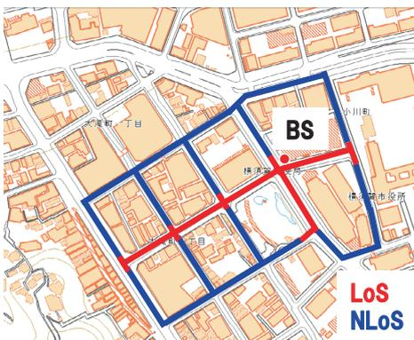
**Fig. 6 Measurement route of MS**
