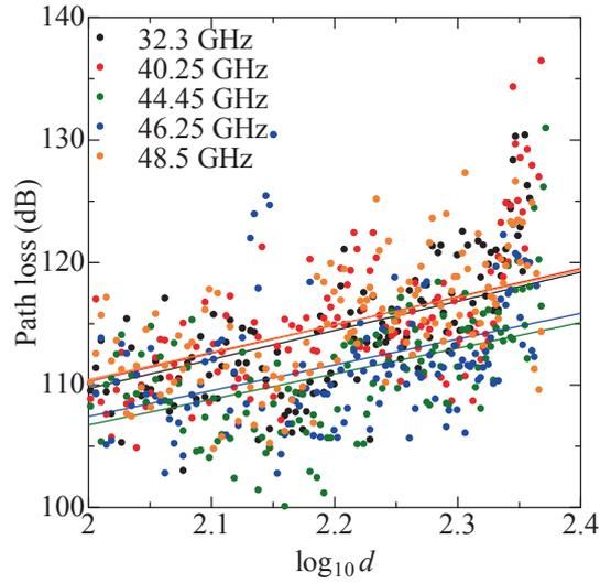
**Fig. 7 Path loss measurement results in LoS urban environment**
