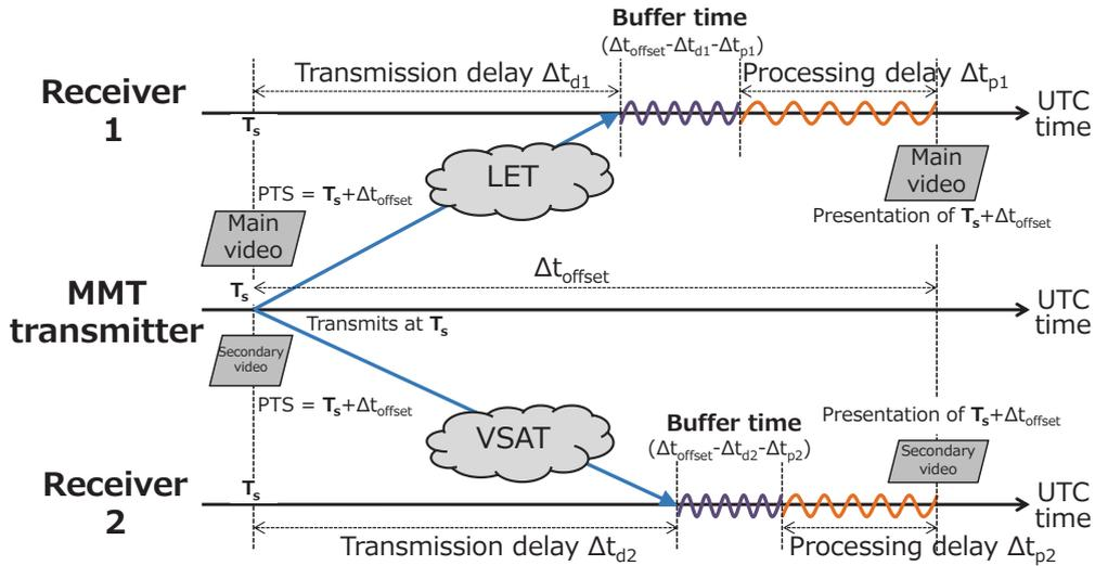
Fig. 1 Mechanism for syncing
