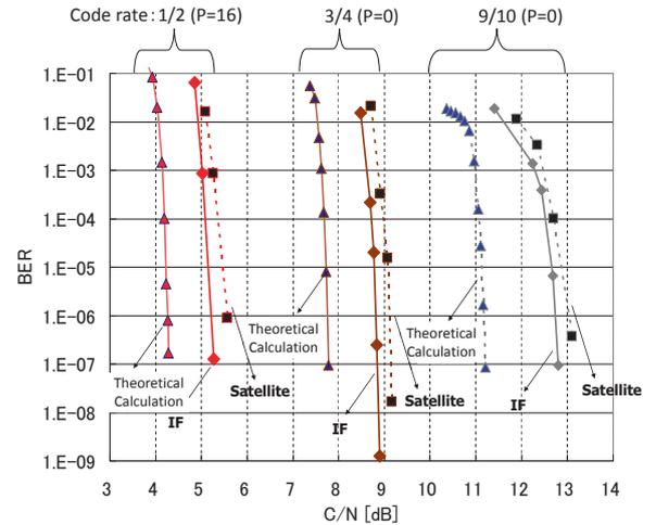
Fig. 10 C/N vs. BER characteristics in WINDS satellite loopback
