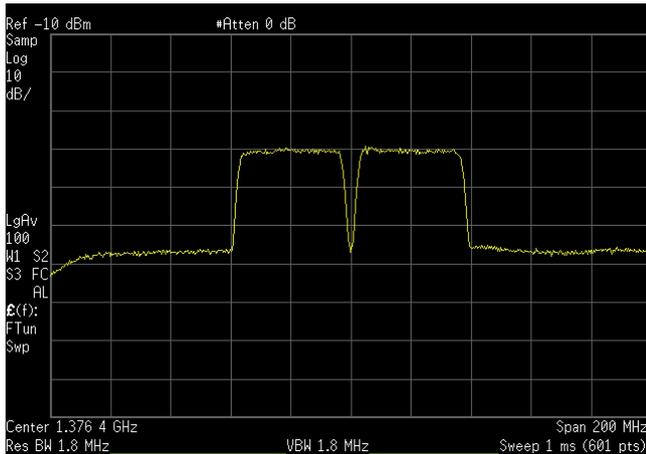
Fig. 4 Reception spectrum (1 GHz band BS-IF signal)
