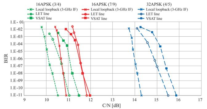
Fig. 5 C/N vs. BER characteristics at WINDS satellite loopback (ISDB-S3)
