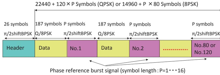
Fig. 8 Phase reference burst signal frame composition
