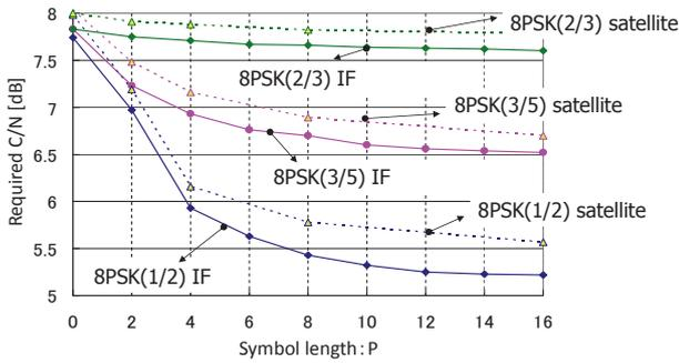
Fig. 9 Characteristics of symbol length vs. necessary C/N
