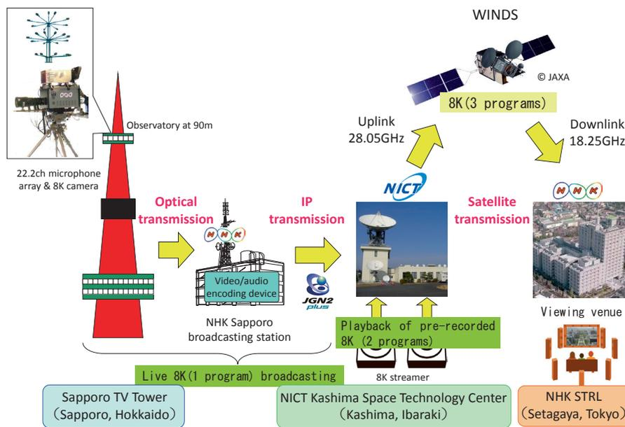
**Fig. 7** Composition of transmission experiments for 8K multi programs (wideband transmission)
