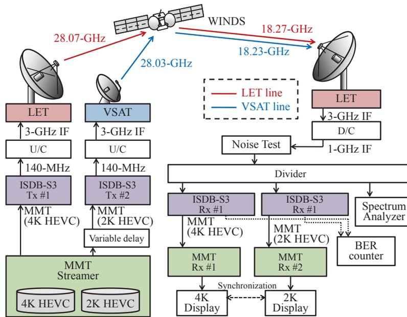
Fig. 2 Composition of WINDS satellite transmission testing (ISDB-S3)
