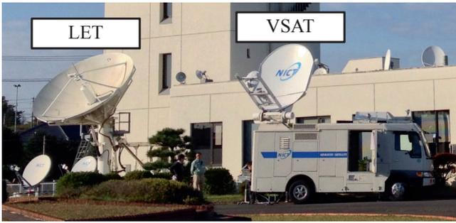
Fig. 3 Exterior of LET and VSAT antenna
