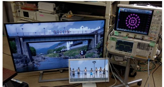
Fig. 6 4K and 2K video synchronization by MMT
