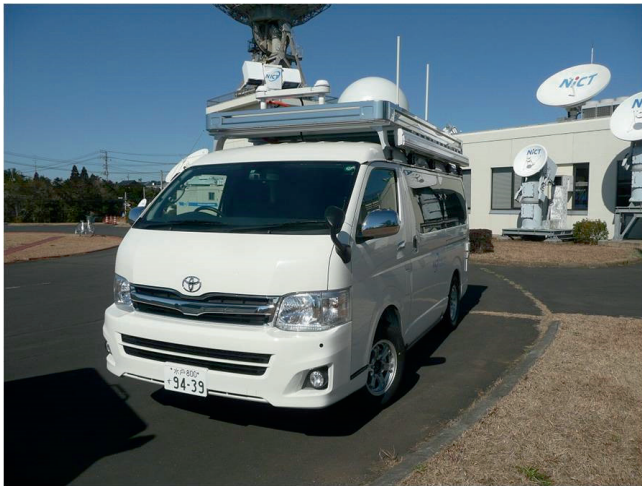
Fig. 1 Appearance of vehicle earth station
