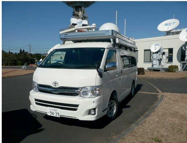
Fig. 1 Mobile vehicle earth station for WINDS
