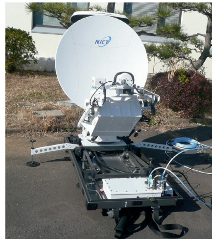
Fig. 2 Fully automatic earth station
