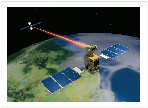
Fig.1 Image of optical inter-orbit communications experiment between the OICETS and ARTEMIS. (The satellite on the near side is the OICETS)
