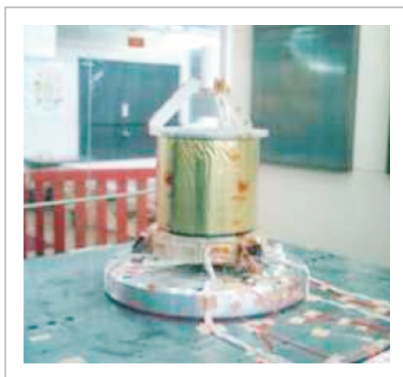
Fig.3 Proof test for optical antenna
