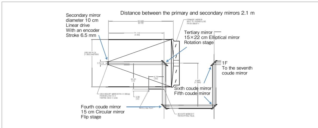
**Fig.3** Configuration of coude optical mirrors
