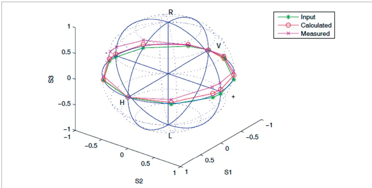
**Fig.6** Measurement examples for the polarization properties of the reflective coating coude mirrors
