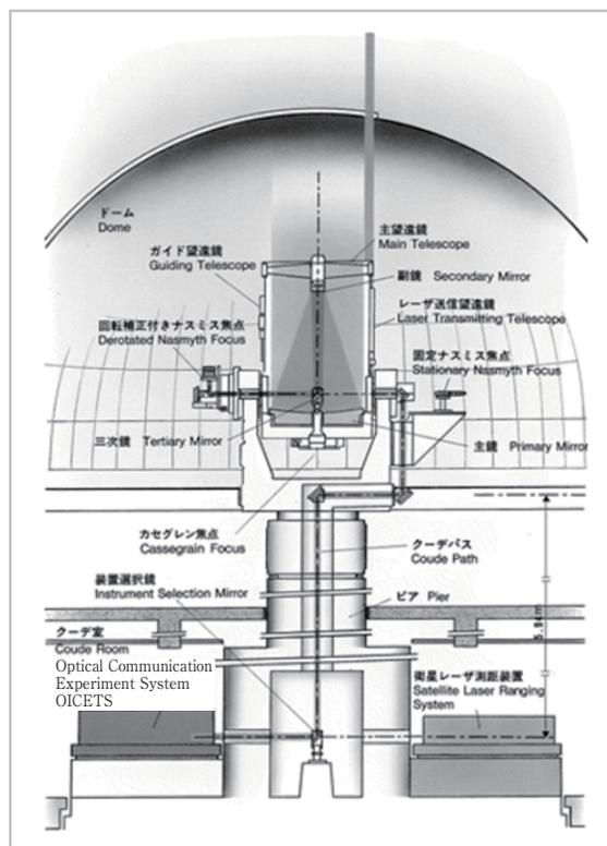
**Fig.1** Configuration of 1.5 m telescope
