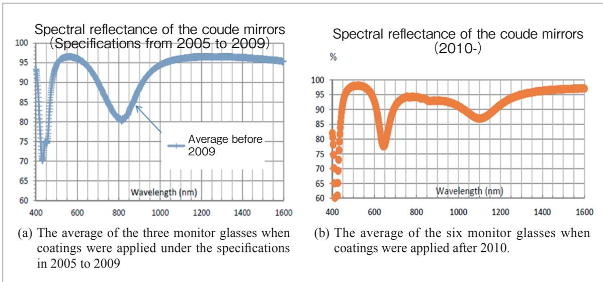
**Fig.5** Spectral reflectance of the coude mirrors
