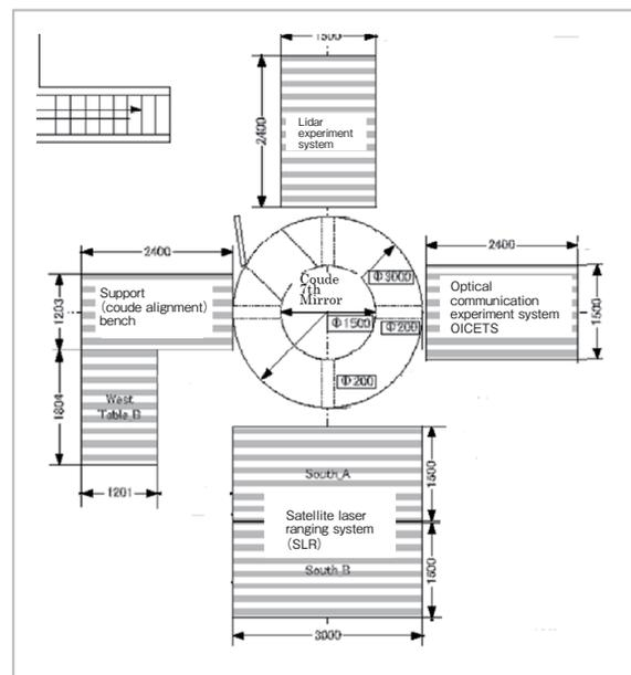
**Fig.4** 1.5 m telescope coude bench
