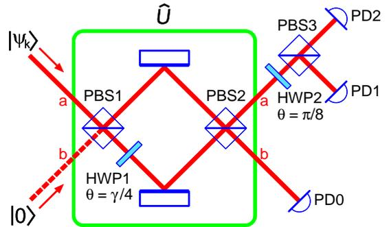
FIG. 4: Principle of the detector that realizes the optimum POM. Here PBS stands for a polarizing beam splitter, HWP for a half waveplate whose axis is rotated by  $\theta$ , and PD for a photodetector.
